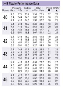
Note: All precipitation rates are calculated for 180 degree operation. For the precipitation rate for a 360 degree sprinkler, divide by 2.
